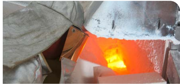
Liquid molten glass in the area encompassing the batch insert of a glass melting tank
