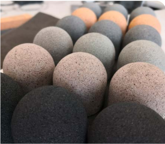
Core sand specimen geometry with various aerogel additives
