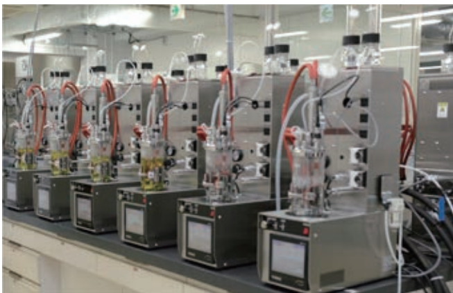
Small-scale fed-batch culture tanks used for validation of practical applications and development of human resources in bioproduction processes
